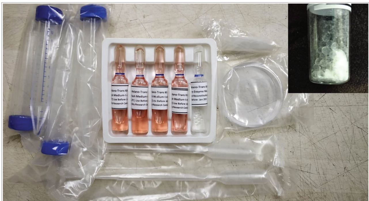
Figure 1: Required chemicals and apparatus for NCES including freeze-dried trypsin coated on silicon pellets (inset)
