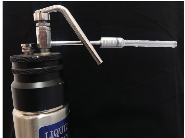
Figure 4: Customized plastic dropper as a disposable extension fitting over the standard straight tip cryocan nozzle
