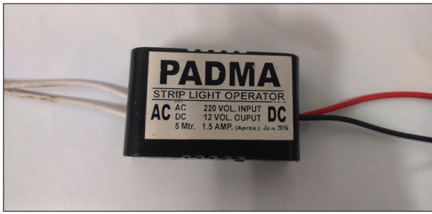
Figure 3: Easily available LED strip light adapter/transformer that converts 220 V/5 A AC current to 12 V/1.5 A DC current
