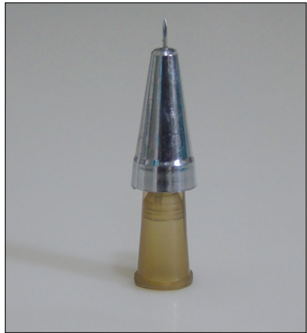
Figure 4: Actual photograph showing combination of needle and tip of the pencil
