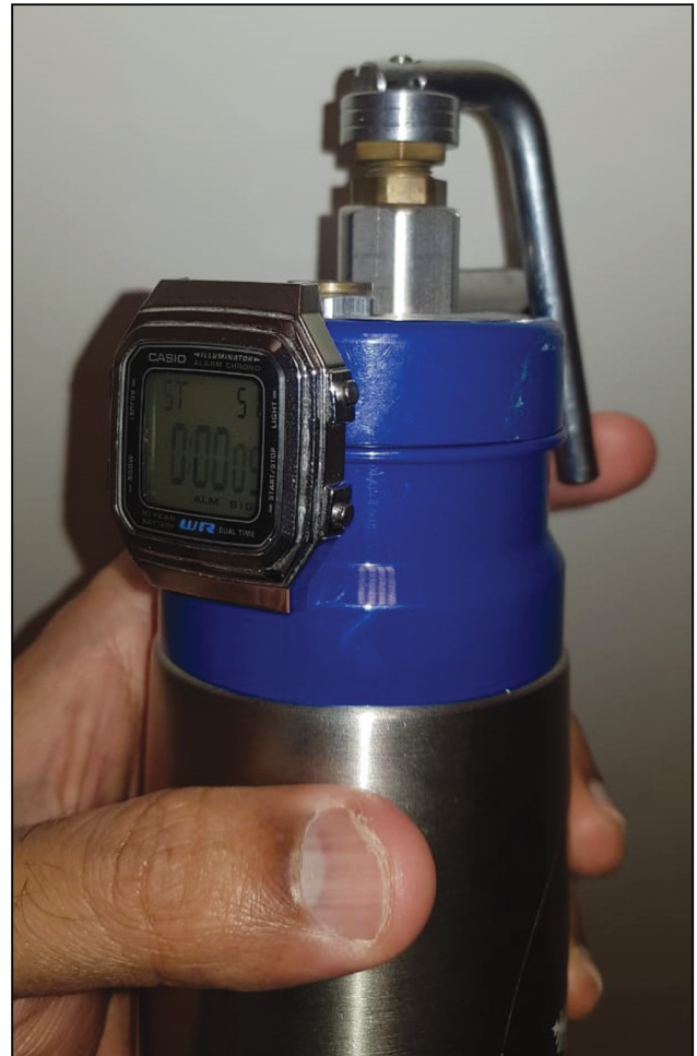
Figure 6: A digital stop watch affixed to the cryogun makes it easy to monitor the correct freeze–thaw timing
