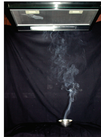
Figure 2: Artificial smoke produced with camphor to show the flow of smoke when the suction is at work
